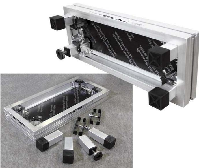
The plywood panel is secured to the frame structure by means of strong adhesive foam, stainless steel screws and silicone, which also contribute to the overall weather resistance of the choral riser.
