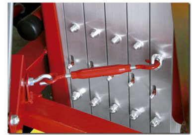
Adjustable mast blocking system for horizontal transportation.
