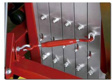
Adjustable mast blocking system for horizontal transportation.
