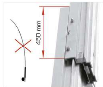
More mast overlap. Prevents fishing rod effect
