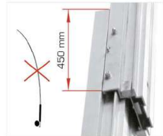
More mast overlap. Prevent fishing rod effect
