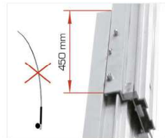
More mast overlap. Prevents fishing rod effect
