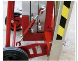
Adjustable mast blocking system for horizontal transportation.
