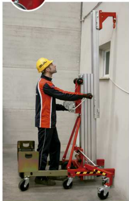
Legs can be inserted in the front or back of the tower for positioning close to walls.
